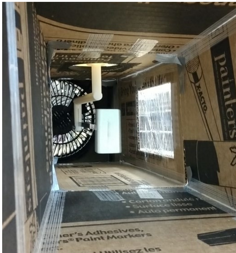
Figure 3. Internal view of the wind tunnel test section with the aeroelasticity experimental setup used to demonstrate a galloping instability.
