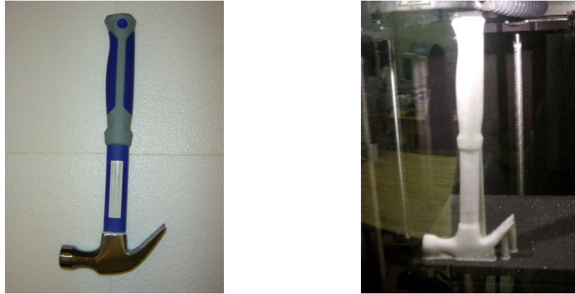
Figure 4. Original and prototype of a hammer inside the build chamber of the 3D Printer
