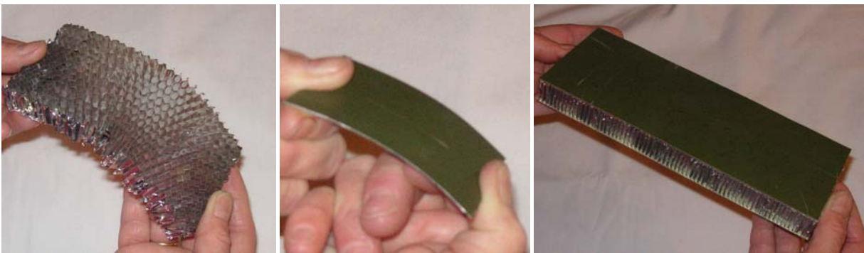
Figure 1. Demonstration of parallel axis theorem: aluminum honeycomb core; aluminum face sheet; sandwich structure
