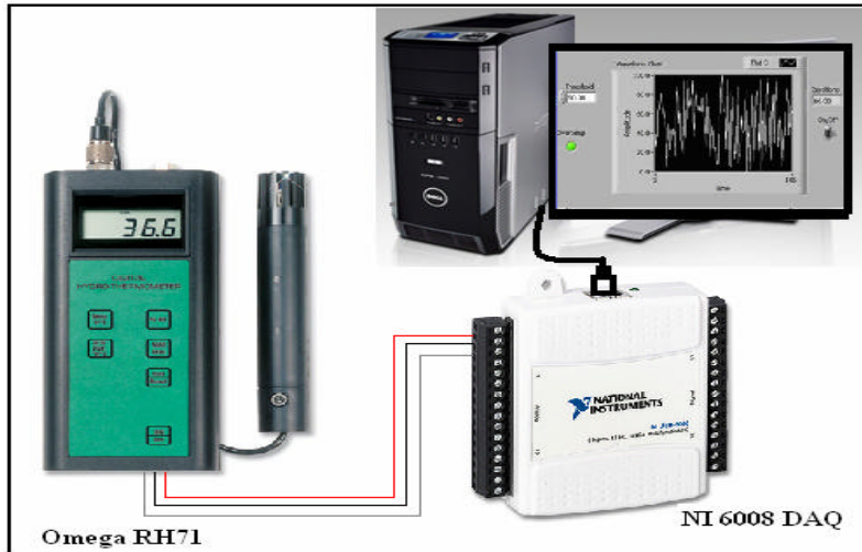
Figure 3: Temperature DAQ Laboratory System Diagram
