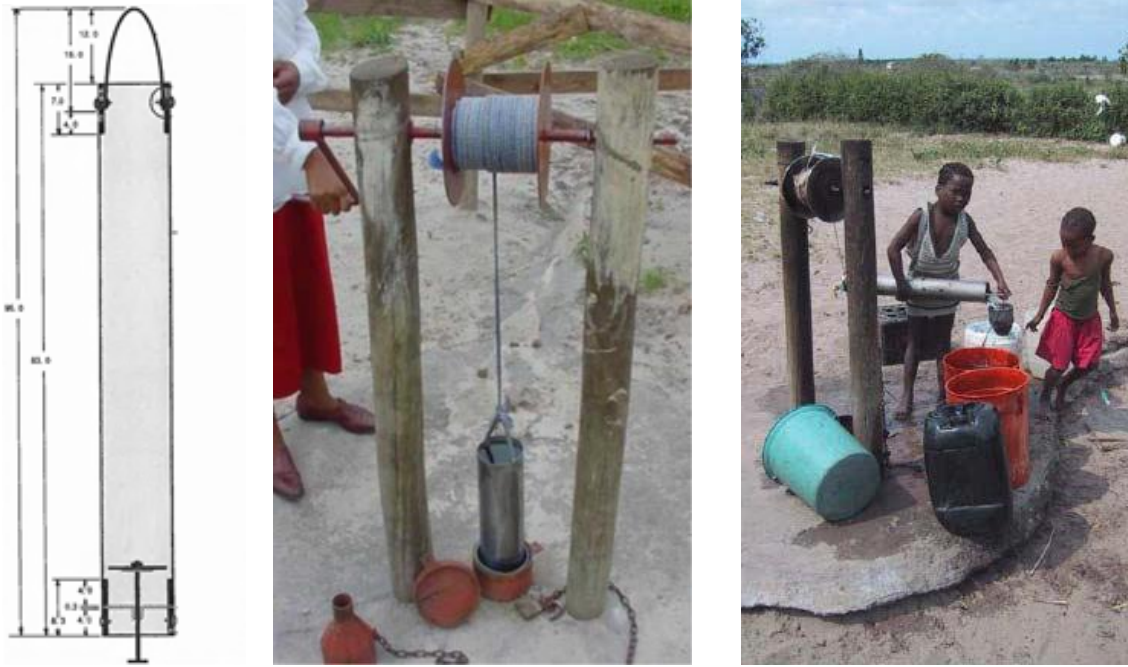
Figure 1 (a) an engineered diagram of a bailer, with a one-way valve at bottom, 5 (b) a bailer being lowered into a borehole in northern KwaZulu-Natal, South Africa, 6 and (c) water from a bailer being emptied into a jerrycan 6
