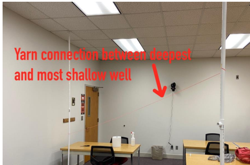
Figure 2: The gradient from the shallowest to the deepest wells is represented by Yarn 1, which connects their respective piezometric head values (marks on the PVC pipes).
