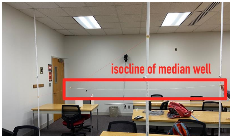
Figure 3: The isocline for the median well ( Yarn 3 ) is represented by a horizontal string which connects the intermediate well's piezometric head value to the same head value on the gradient line ( Yarn 1 , which connects the deepest to shallowest wells).
