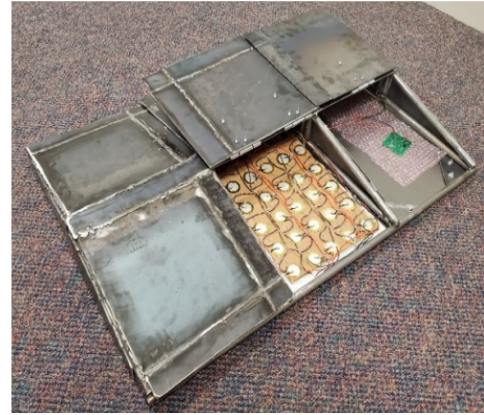
Figure 7: Final casing with piezoelectric network installed with charging circuitry.
