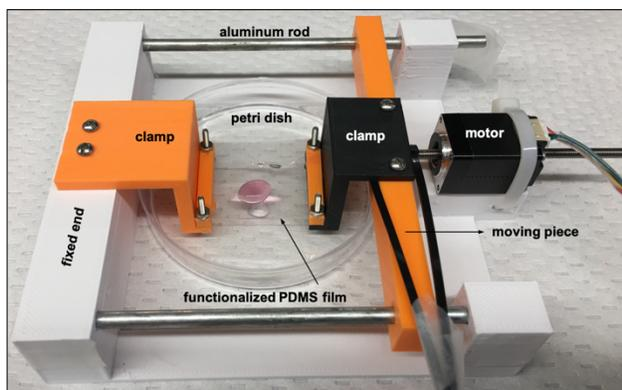
**Figure 5:** Final assembly of the main frame with motor.
