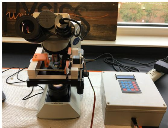
**Figure 8:** Stretch chamber on the microscope stage and connected to the control unit.
