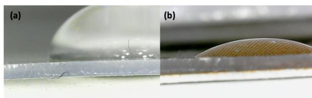
**Figure 4:** Contact angle of water (a) before and (b) after oxidation of PDMS surface.
