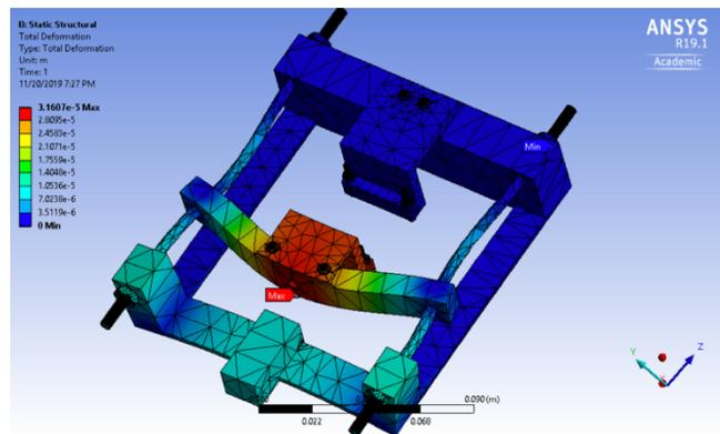
Figure 7: Finite element analysis results for deformation. The maximum deformation occurs at the middle of mobile piece.
