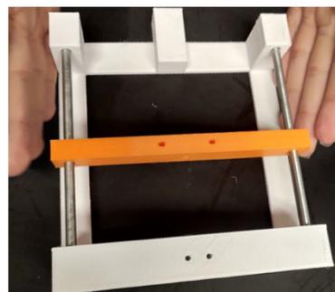
**Figure 3:** 3D printed main frame with rods and moving pieces.
