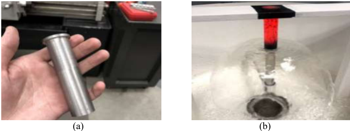
Figure 5. Jominy end-quench specimen: manufactured standardized specimen (a); standardized quenching of the test specimen (4140 steel)
