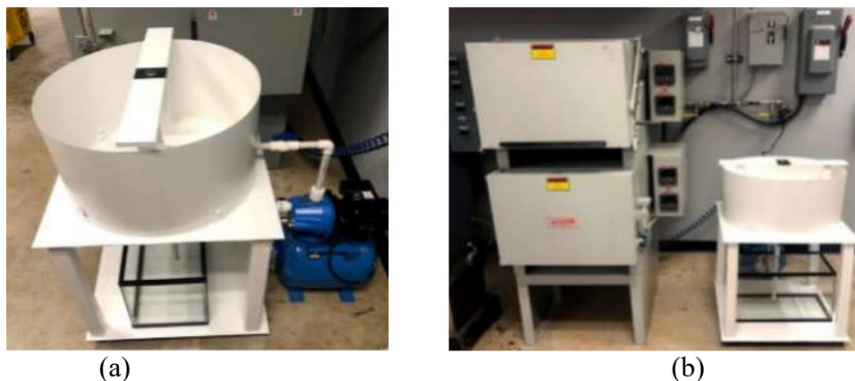
Figure 4. Completed Jominy end-quench tester (a); placement of the tester adjacent to the laboratory furnace (b)
