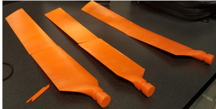
Figure 13: Baseline pin locking mechanism replica of Wind Turbine Technologies turbine blade
