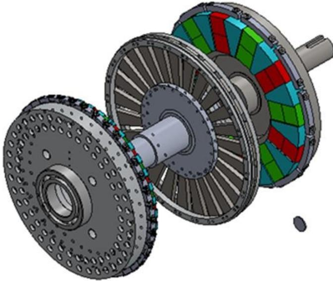
Figure 1. Example of an axial-flux-focusing magnetic gear, showing a low speed rotor, spoke rotor, and high speed rotor. Green and red correspond to magnets of opposite polarity in this figure.
