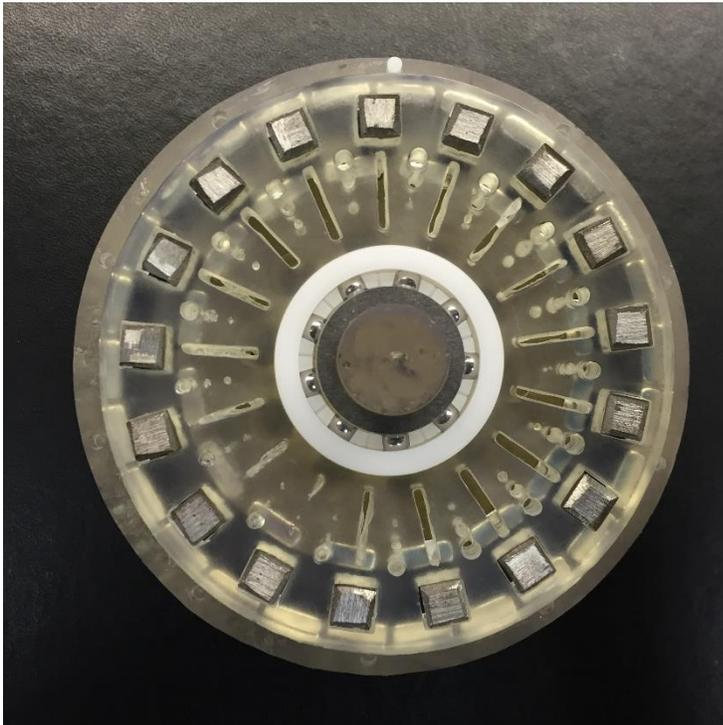
Figure 9. The radial-flux-focusing magnetic gear partially assembled showing the optical clarity through the cage rotor plate following fine polishing, allowing visualization of both the inner and outer rotor magnets.
