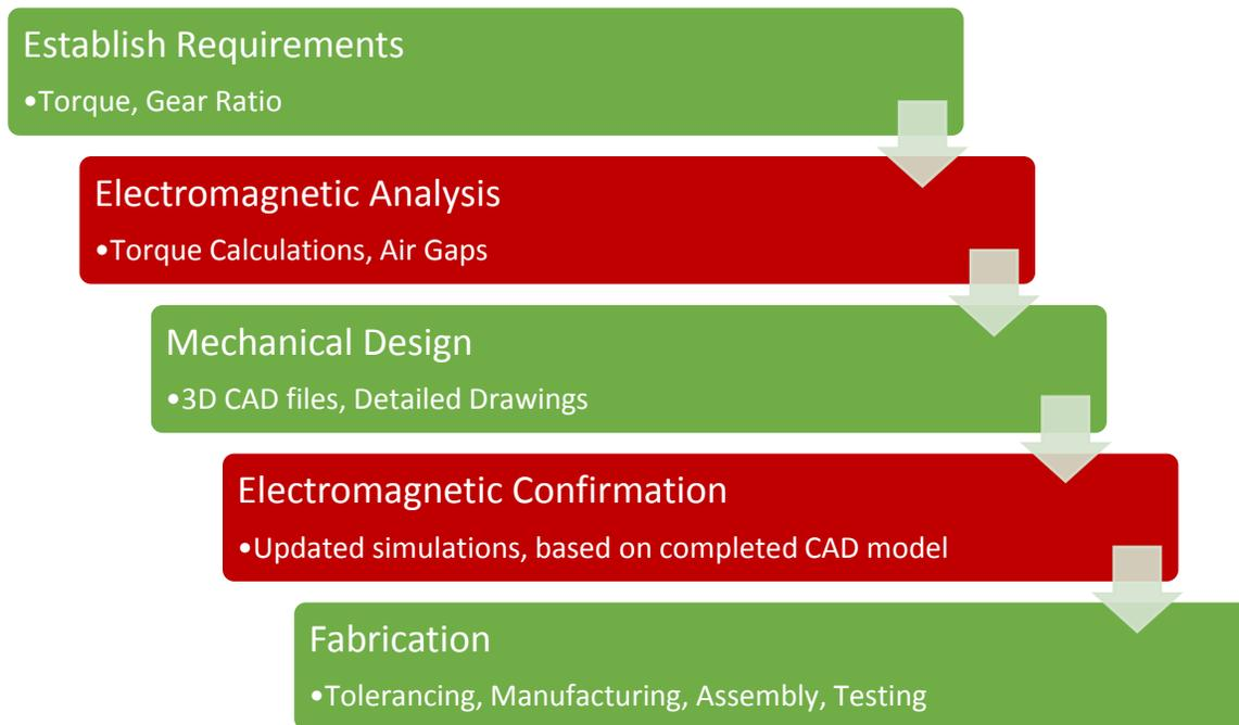
Figure 3. Magnetic gear design process, with primarily mechanical/manufacturing stages shown in green and primarily electromagnetic stages shown in red.
