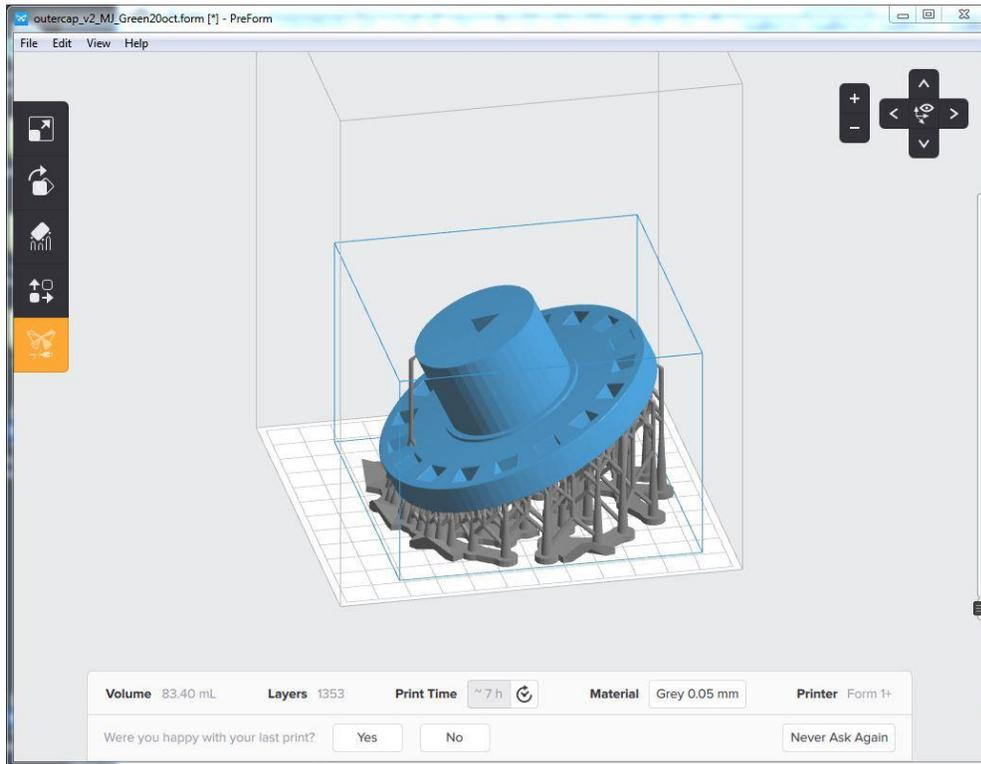
Figure 6. Screenshot of the PreForm software showing part orientation and the generated support structures.
