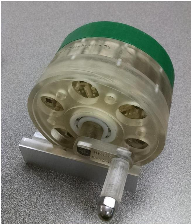
Figure 10. Completed radial-flux-focusing magnetic gear assembly.
