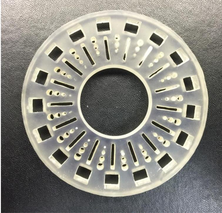
Figure 8. Cage rotor plate manufactured from Clear Resin after wet sanding to translucence.
