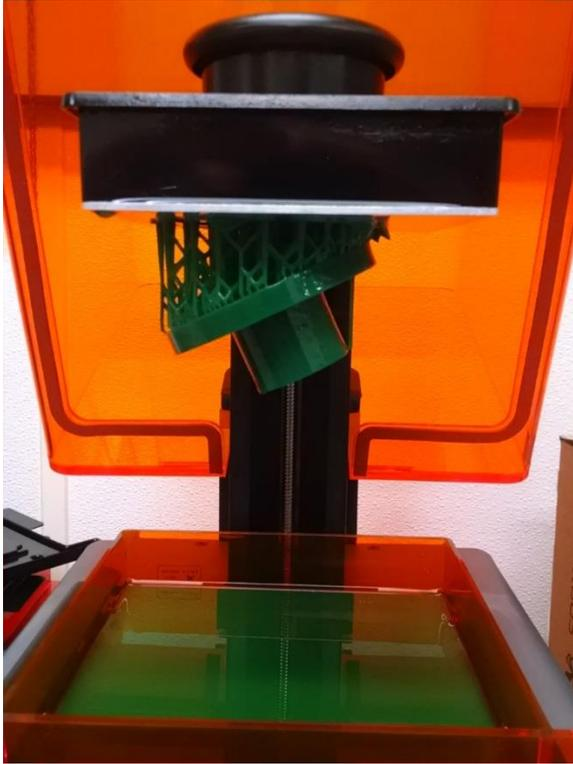
*Figure 7. The cage rotor output shaft (in Maker Juice SF Green) immediately after fabrication on the Form 1+, inverted and attached to the build platform via scaffold structure.*
