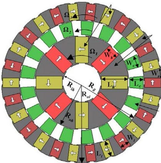
Figure 2. Example of a radial-flux-focusing gear, showing the outer rotor, cage rotor, and inner rotor<sup>2</sup>. Red and gold correspond to magnets of opposite polarity in this figure, with green representing the steel flux focusing pieces.
