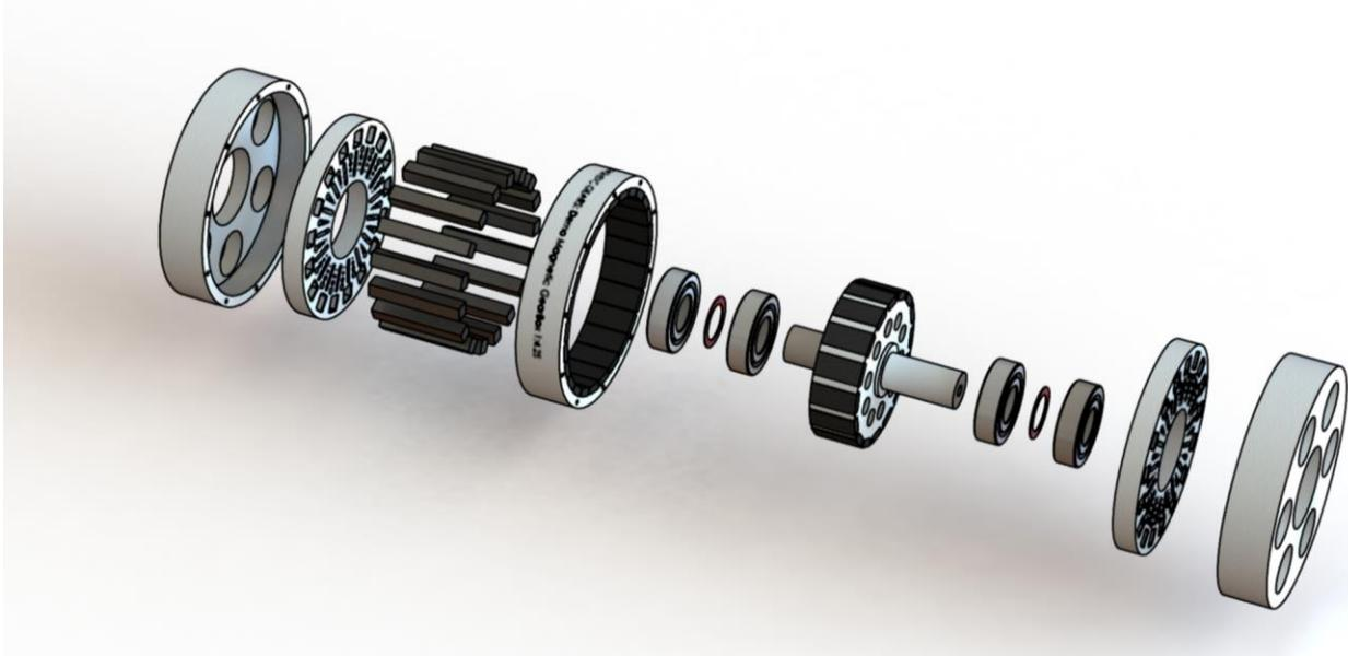
Figure 5. Solidworks exploded assembly view of the radial-flux-focusing magnetic gear.
