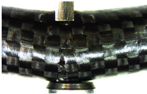
(Figure 13. Carbon-fiber at end of testing)
