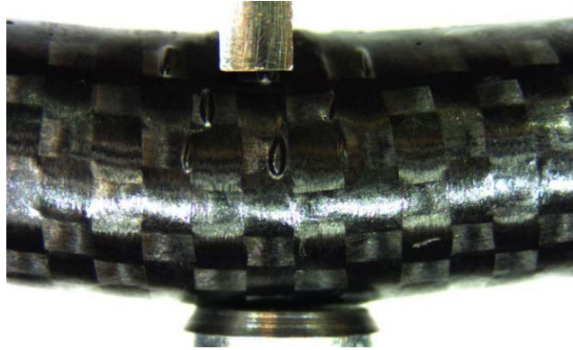
(Figure 12. Carbon-fiber during testing)
