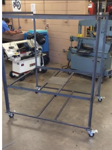
Figure 10: Completed test section frame.
