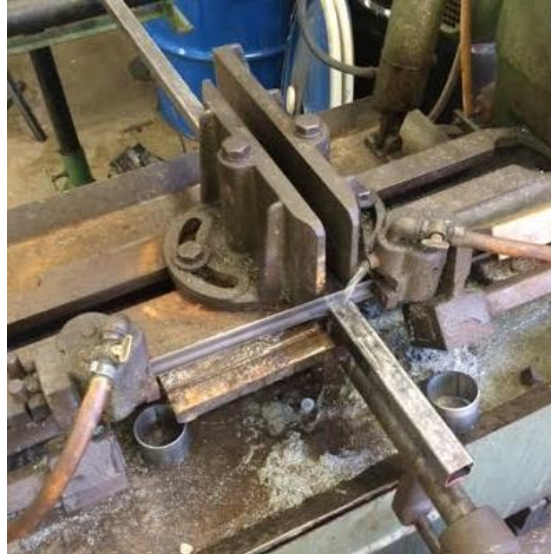
Figure 8: Cutting material with horizontal band saw.
