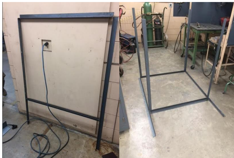
Figure 9: Construction of angle steel frame.
