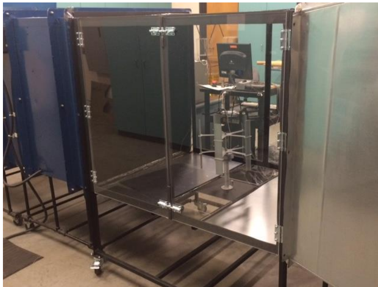
Figure 11: New test section installed with existing wind tunnel.
