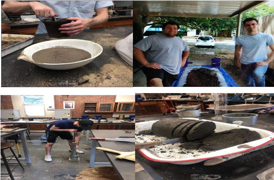
Figure 1. (top left) dry sample of Pluff Mud, (top right) moist sample of Pluff Mud, (bottom left) Undergraduate researcher is performing the standard Proctor test, (bottom right) compacted sample of Pluff Mud.
