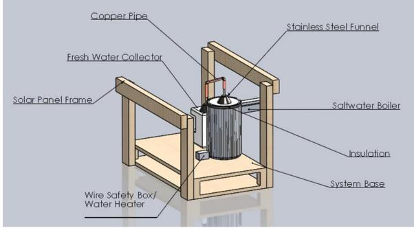
Fig. 2: Basic solar powered desalination plant.
