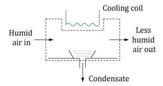
Fig. 3: Schematic of a dehumidification process (see Moran et. al<sup>4</sup>).
