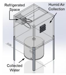
Fig. 4: Solar powered water collection via dehumidification.
