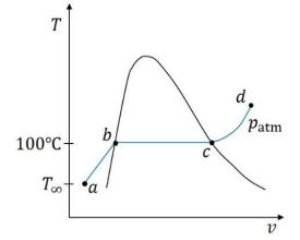
Fig. 1: T-v diagram for the vaporization of water at constant pressure (see Moran et. al<sup>4</sup>).
