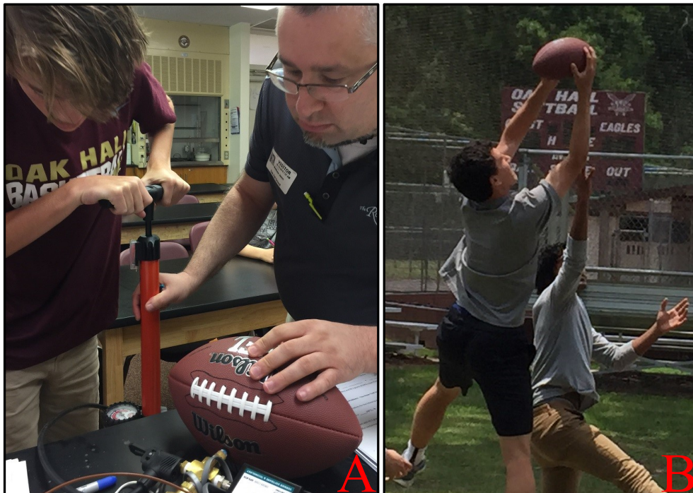
Figure 1: (A) With instructor guidance, a chemistry student hand-inflates a game football to regulation pressure under ambient classroom conditions in preparation for a cold soak in the school freezer. (B) To simulate game play at a different ambient temperature than where the ball started, students scrimmaged with the cold-soaked football for 20 minutes to warm it up.
