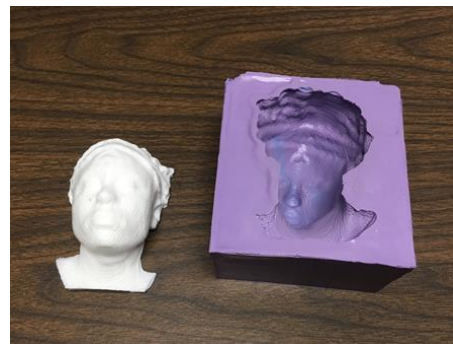
Figure 5: Silicon mold and acrylic casting
