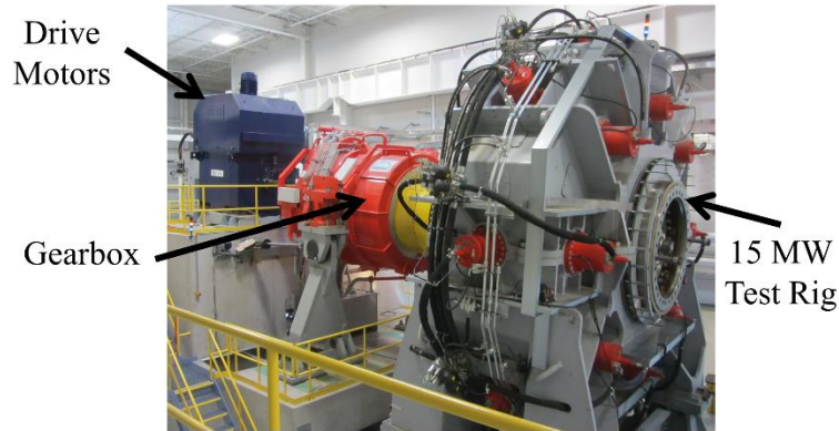
Figure 1. Clemson 15MW wind turbine test platform
