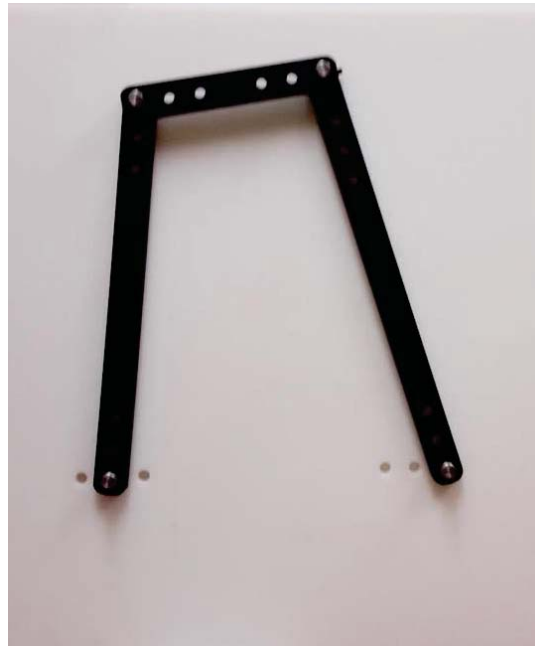
Figure 2. Adjustable 4-bar mechanism used in pilot study.
