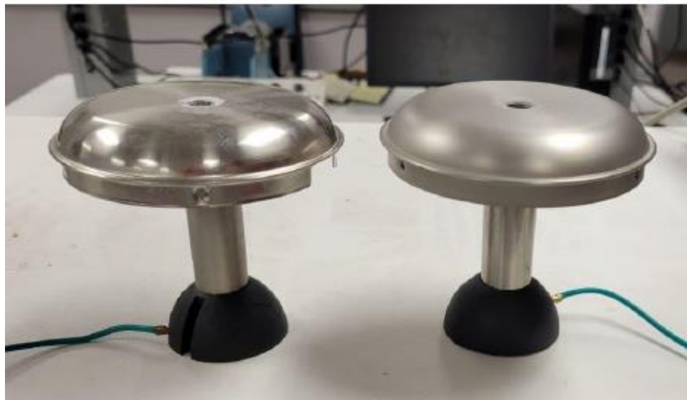
Figure 5. Ceiling-fan shafts as antennas (courtesy of Jonathan Dobson-Lewis, Summer 2021).
