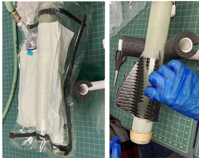
Figure 2. Tip-to-tip carbon fiber reinforcing for the rocket fins done in the materials laboratory.
