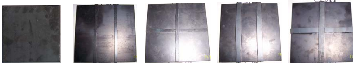
Figure 9. The Specimens Used in the 2^2 Factorial Experiments. From Left to Right: Smooth plate, Small-rib-parallel plate, Small-rib-cross plate, Big-rib-parallel plate, Big-rib-cross plate,
