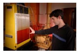
**Fan performance lab** (Plint & Partners, original cost approximately \$20,000) – In this lab, students measure the head gain at various flow rates, and rpm's and torque of a fan. Using the data, students develop a fan performance curve which is used to determine the correct size of a fan or pump for a given piping system. Head gain and flow velocity are determined by measuring pressure with a manometer consisting of a bank of tubes.
