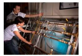
**Pipe loss experiment** (constructed in-house, approximately \$10,000) – In this experiment, students measure the head loss due to friction in selected pipes and fittings at different flow rates. From the data, students determine friction factors. Flow rate is measured using Proteus electronic flow meters integrated with Labview. Head loss is determined by measuring height of water in tubes with a tape measure.
