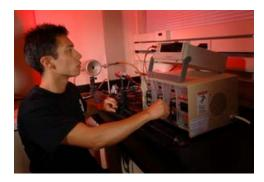
**Radiation Lab** (constructed in house, approximately \$10,000) – In this lab, students measure the radiative heat transfer from an oven at various distances. By comparing the measurements with theoretical predictions, students can determine the emissivity of the oven as well as the performance of the detector.
