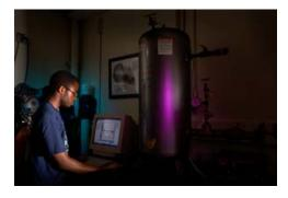
Tank discharge lab (constructed in house. approximately \$10,000) - Students learn the principles of compressible flow, and they develop the theory of a choked orifice flow meter. Pressure and temperature are measured in a large tank at one millisecond intervals using an electronic pressure transducer and thermocouple connected to a computer. Mass flow rate is calculated, and comparisons are made between theoretical calculations and measured values.
