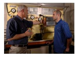
**Air conditioning lab** (Technovate Air Conditioning and Refrigeration Lab, approximately \$27,000) - In this lab, students learn the thermodynamics of the various refrigeration cycles. By measuring temperature, pressure, and flow rates at various points in the cycle, students calculate the performance and power requirements of an air-conditioner. Students manually record the temperature and pressures at the different state points.
