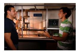
**Heat Exchanger Lab** (constructed in house, approximately \$15,000) – In this lab, students analyze a concentric double-pipe heat exchanger by measuring inlet and outlet temperatures of the two fluids as well as their flow rates. From this information, students calculate the heat flux and overall heat transfer coefficient.
