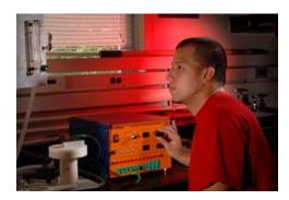
**Heat Conduction Lab** (HT10XC-B Heat Transfer Service Unit, HT11 Linear Heat Transfer, HT12 Radial Heat Transfer, \$23,601) – In this lab, students are taught the principles of linear and radial heat conduction and how to use that theory to measure heat flux. They learn how to find contact resistance and how to determine the thermal conductivity of various materials. Thermal circuit diagrams are emphasized.
