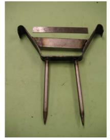
Figure 3. Welding shop practical exam: boot scraper
