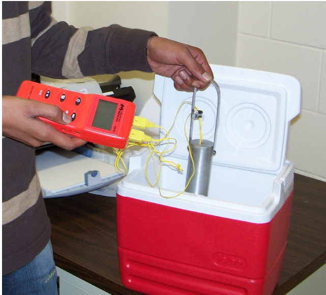
Figure 1. Immersing aluminum cylinder in iced-water experiment
