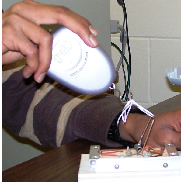
Figure 4. Twisting the mousetrap spring experiment
