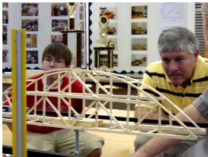
Figure 1- Model Bridge on the test stand with the loading attachments
