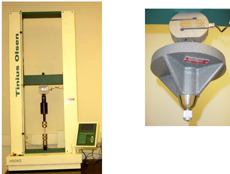
Figure 1. Universal Testing Machine and Brinell hardness attachment connected to the Load Cell
