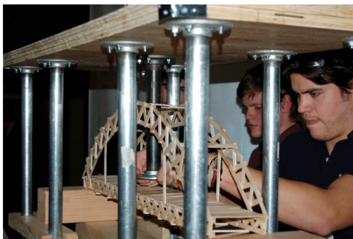
Figure 3: Load test of a bridge. ASCE student members Kalen Bauman (left) and Alejandro Prieto (right) pictured.
