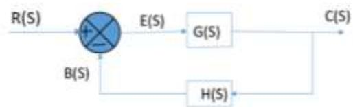
Figure 2: Block diagram of a closed loop control system
