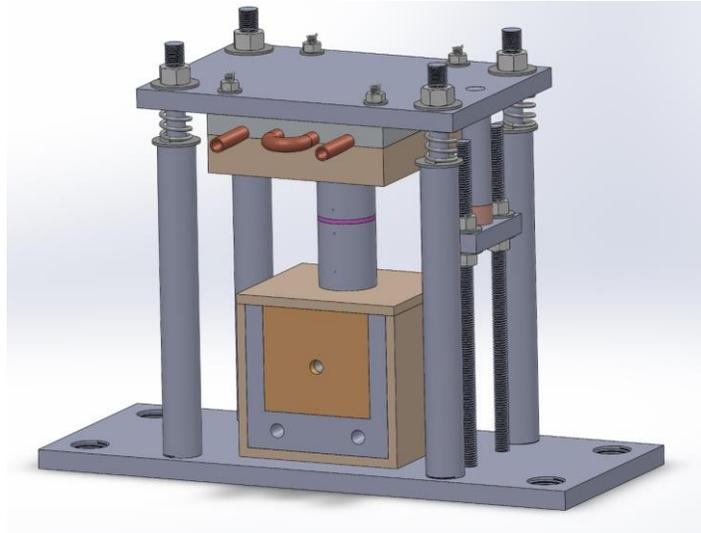
*Figure 7. The inner housing consists of an aluminum base plate with four identical aluminum bars supporting an aluminum top plate that is mounted to the cold plate using nuts and bolts. Springs rest on the stepped portion of the support bars and support the top plate. Two threaded rods on the right side of the inner housing support the load cell which rests on top of an adjustable height platform.*
