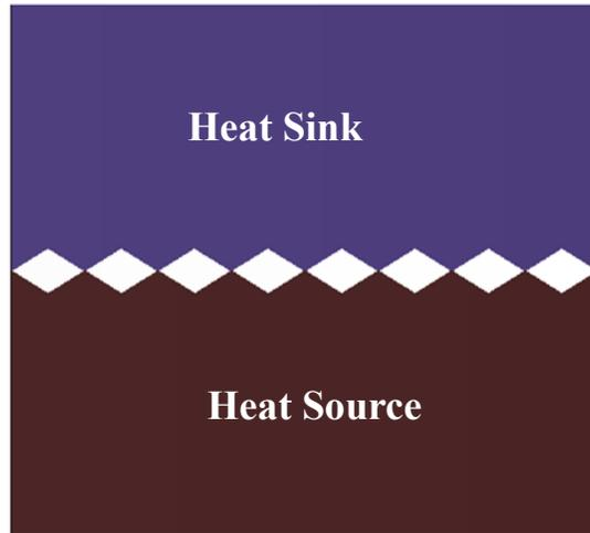
*Figure 1. An imperfect mating surface is created by the roughness of the heat source and heat sink. As a result, air pockets with low thermal conductivity develop and prevent effective heat transfer.*
