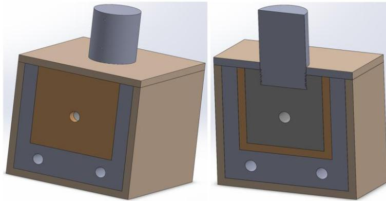
*Figure 6. The heater block assembly employs cartridge heaters to heat the central block and guard heater blocks while insulating wood paneling ensures all of the heat generated passes through the meter bars. Piping insulation around the meter bars is not shown.*
