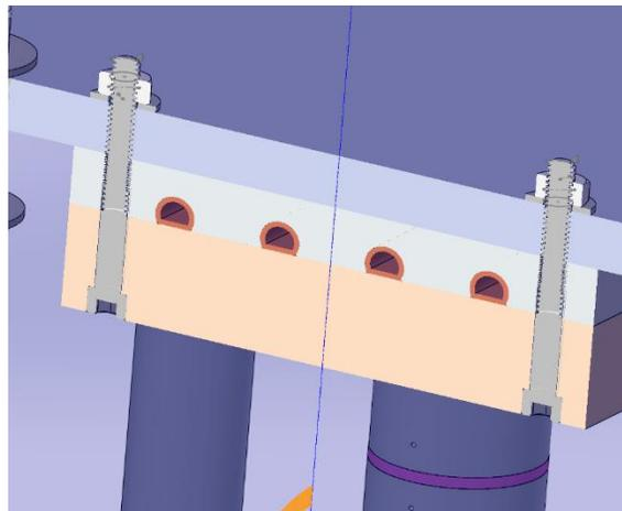
*Figure 8. Cross section of the aluminum plate-cold plate-wood block fastened assembly. This design avoids compromising the cold plate tubing, and the top meter bar can be moved freely up and down as the support bar springs compress and extend.*
