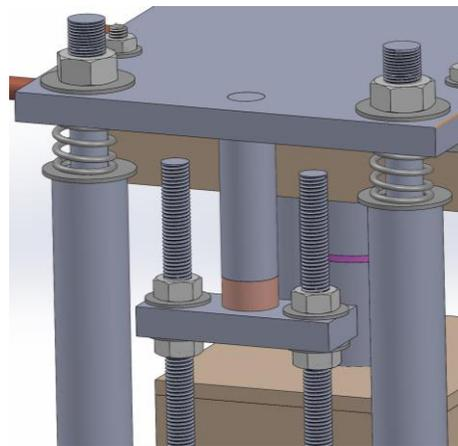
*Figure 9. The load cell (small brown cylinder) is compressed by an aluminum bar that is threaded and screwed into the bottom face of the middle plate. The threaded rods and nuts allow the height of the load cell to be adjusted when different thickness TIMs are tested.*
