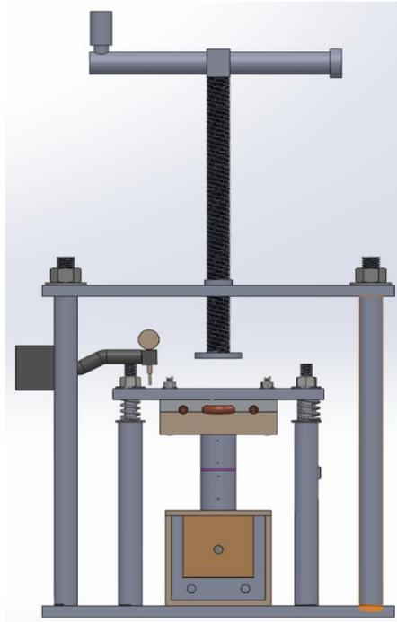
*Figure 4. Front view of the final design. The screw press applies a compressive force onto the inner housing which compresses the TIM. Springs located in-line with the inner housing support bars return the top plate of the inner housing to its original position.*
