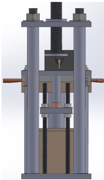
*Figure 5. Pressure is recorded by a load cell (small brown cylinder) that is supported by an adjustable-height platform. The load cell button is compressed by an identical diameter bar*
