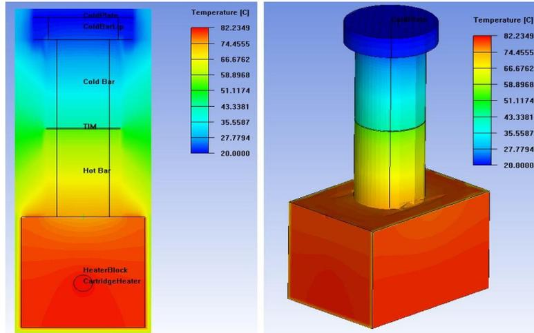
*Figure 11. IcePak model results. The first thermocouple must be placed at a minimum height of 2.5cm from the bottom face of the hot meter bar in order to linearly extrapolate the temperature at each TIM interface. The first thermocouple will be placed at a distance greater than this as a design “safety” factor to ensure the thermocouple is in a zone of uniform heat flux.*
