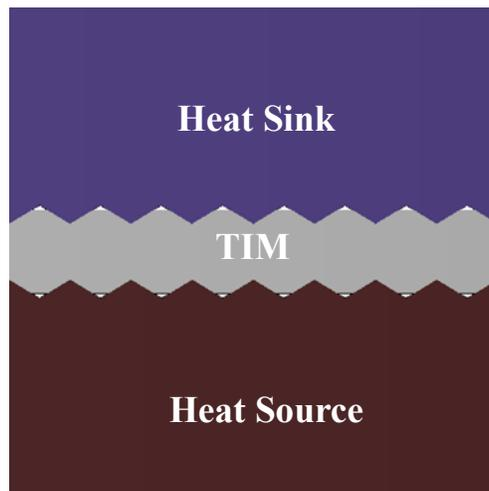
*Figure 2. The ideal TIM possesses a high thermal conductivity and can deform to fill in any air pockets.*
