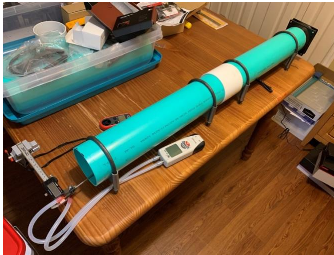
Fig. 2. Velocity profile interrogator kit setup reflecting the conditions a remote learner may experience.
