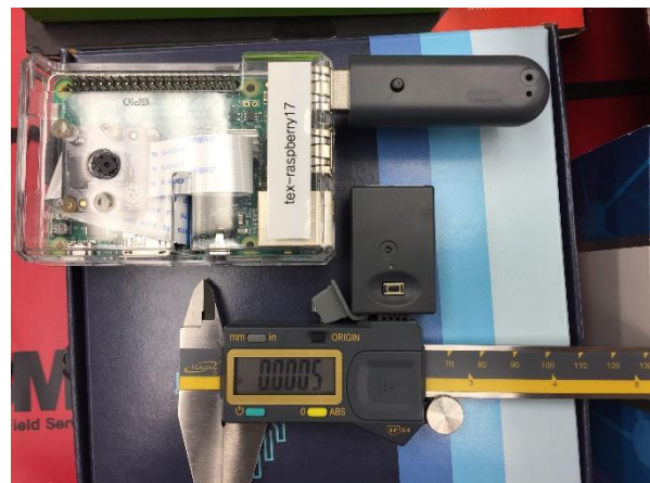
Figure 3: Raspberry Pi with magnetic card reader and wireless caliper
