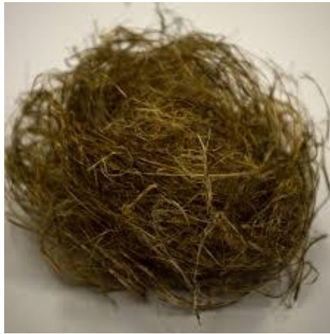
Figure 1. Sunstrand hemp fiber treated for composite application.
