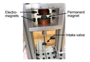
The permanent magnet at fixed to the shaft of the intake valve. The permanent magnets have reverse polarity, and are turned on and off by a signal from a computer that is synchronized to the engine speed. The electromagnets cause the permanent magnet to "pop off" the iron core of the electromagnets and move to the opposing side. The rpm and power of the engine is determined by how long the valve is open on the intake stroke of the engine.
