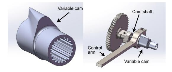
As shown in the figure above, the variable cam slides along the splined cam shaft. In the figure above on the left, an enlarged view of the variable cam is seen.
