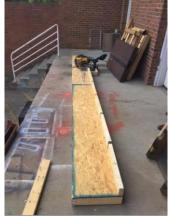
Figure 2: De-nailing jig
