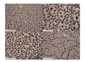
Figure 3: Optical microscopy images of titanium coated epoxy after 0, 300, 600 and 1200 hours of exposure (500 X magnification)
