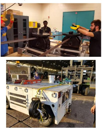
Figure 2. Top: G-Loading test shows temporary deflection after 778 lbs. were placed on top of the rig at the Structures Lab in the CoE. Bottom: Final structural G-load test at Ellington Field with AOD team.
