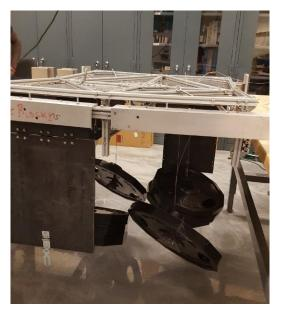
Figure 1. G-Loading test shows temporary deflection after 370 lbs. were suspended from the rig at the Structures Lab in the College of Engineering (CoE).
