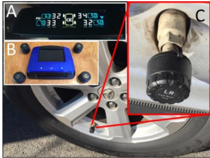
Figure 2: An aftermarket Tire Pressure Monitoring System (TPMS) was installed on a test vehicle to measure tire temperature when driving with one tire underinflated. Inset A shows the cabin display from which TPMS data were collected while driving. Inset B shows the wireless caps and solar-power receiver before installation. Inset C is a close-up of one TPMS cap installed on a tire’s Schrader valve stem.
