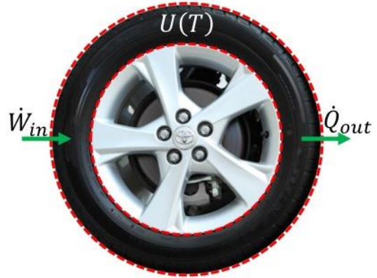
Figure 3: A closed system is established upon a car tire, enabling a First Law energy balance. The tire absorbs mechanical power from its surroundings, warms up, and releases heat back to the environment. In steady state, absorbed mechanical power matches outwardly convected thermal power, and the tire's temperature remains fixed.
