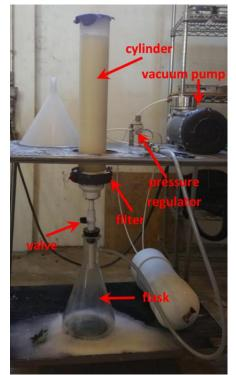
Figure 2. Batch filtration experiment.
