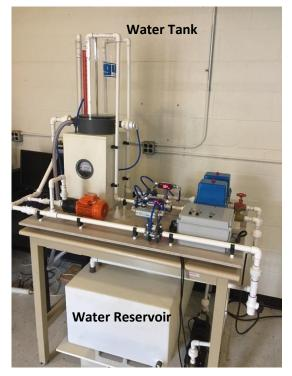
Figure 1. Water tank experiment. Pumps circulate water from bottom reservoir (below table) to tank above.
