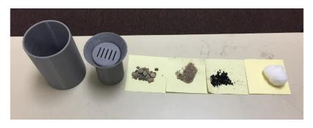
Figure 2: Prototype of 3d Printed Smart Cup (cup, filtering cartridge, and lid) and filtration materials (gravel, sand, granular activated carbon, and cotton wool).
