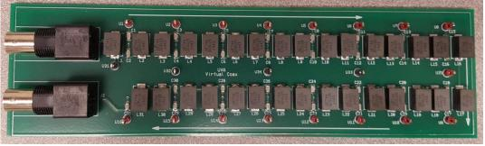
Figure 2 Artificial Transmission Line
