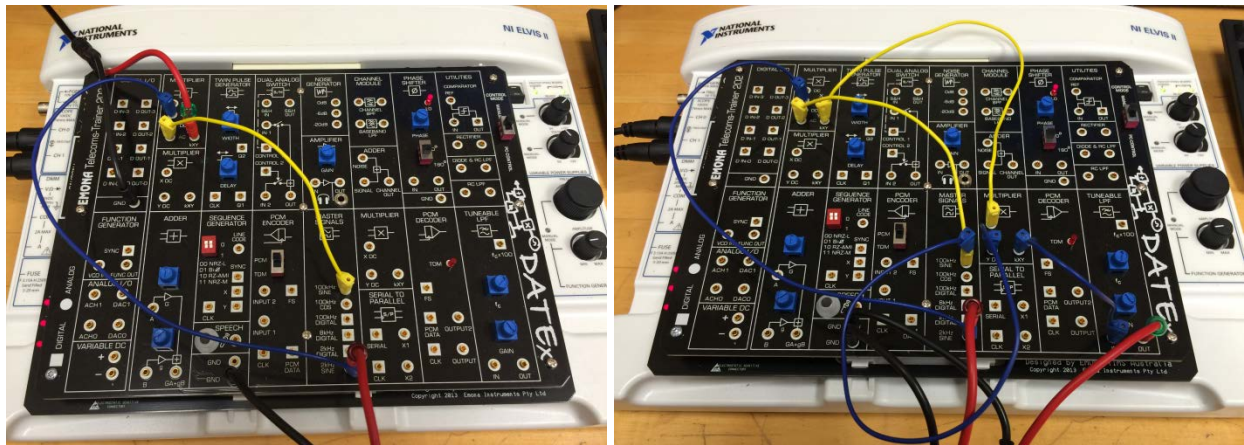
Figure 7- Physical Setup for DSB-SC (a) Modulation (b) Demodulation
