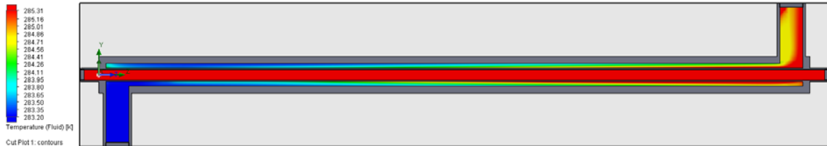
Figure 7. Temperature Profile of Shell Fluid in Parallel-flow Arrangement
