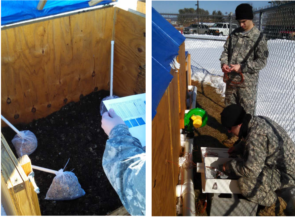
Figures 3 and 4. Samples stored in laundry bags and access tube to take samples. CE cadets attach thermocouples to the data acquisition system.
