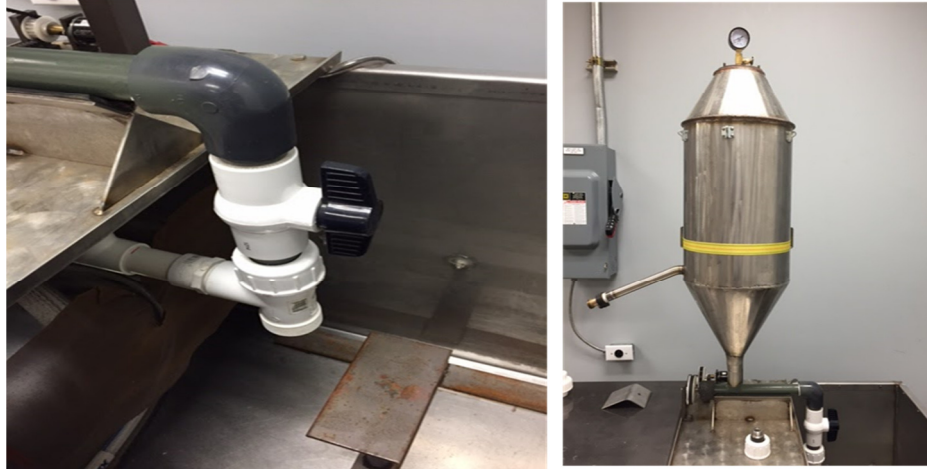
Figure 3: Manifold from Hopper to Nozzle
