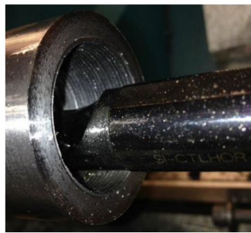
Figure 3: Internal Threaded on Lathe
