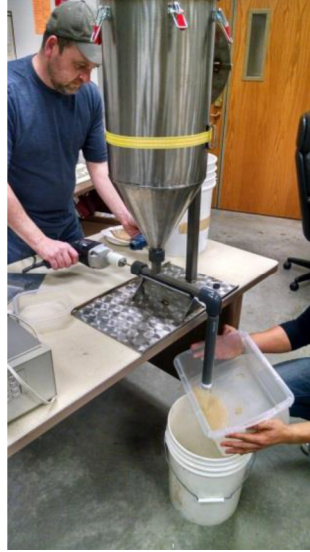
Figure 9: Sand Flow through Auger System Test
