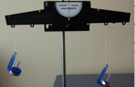
4) The fourth demonstration involved an equal arm balance with an angle indicator on it. As a demonstration of the law of the lever, students were asked to show that the weight times the distance on the left matched the weight times the distance on the right. Students were then shown an unequal (not level) condition and asked to calculate what would be necessary to add to return the system to equilibrium. Class time spent: about 5 minutes.
