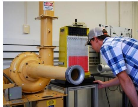
*Figure 1b. Blower Housing in test rig*
