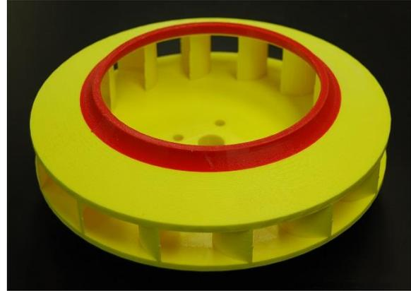
Figure 3b. Impeller prototype made of ABS plastic, designed and printed by one of the student teams.
