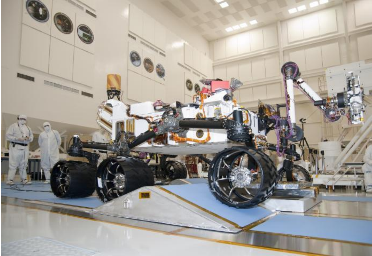
Figure 1. NASA's next Mars rover, Curiosity, drives up a ramp during a test at NASA's Jet Propulsion Laboratory, Pasadena, Calif., on Sept. 10, 2010 2
