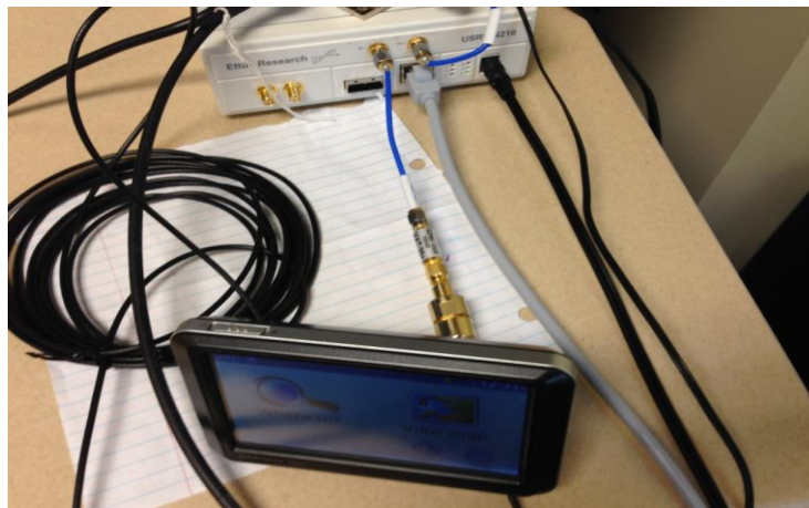
Figure 4 Testbed setup with the GPS receiver and the USRP.
